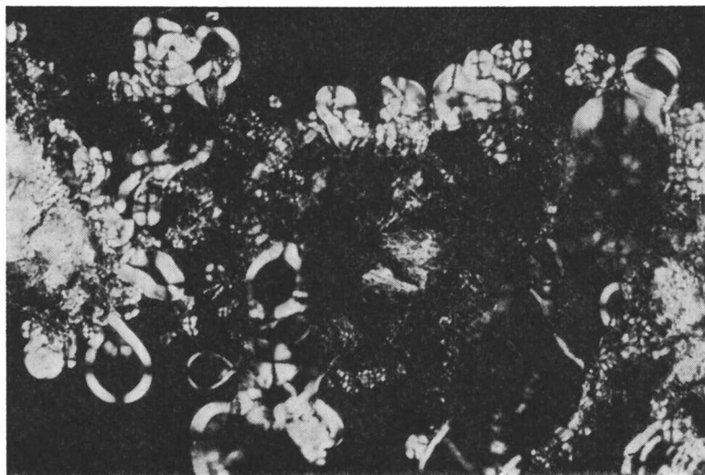
Figure 5. Solid crystal of cholesterol forming spherulitic mesophase with a polyoxyethylene ester (Tween 40) in water Polarized light \times 100
